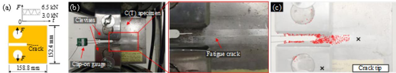
Figure 1. (a) Schematic of the test setup; (b) photo of the test setup.  $F$  is the applied fatigue load cycles and  $t$  is time; and (c) fatigue crack localized by a set of highlighted pixels. (3)
