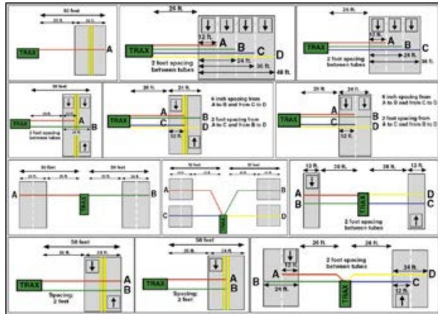
Figure 2. Pneumatic Road Tube Layout Samples (2)
