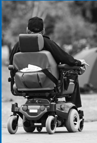
Not all wheelchairs and scooters have traditional frame joints that can accept vehicle tie-down devices.
