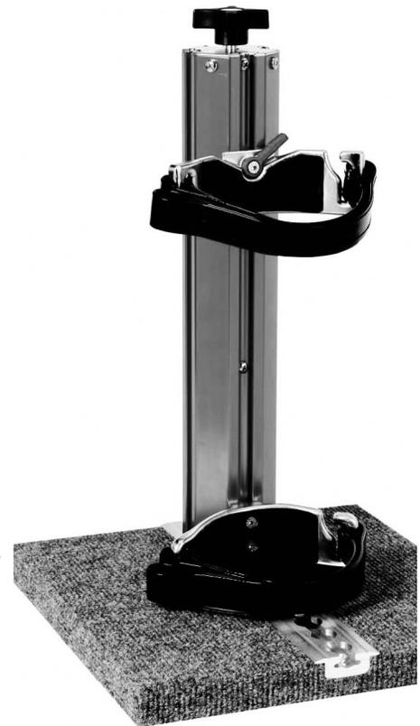
*The GO2, above, locks into the L-track the same way a wheelchair securement retractor slides into place. Install the track fitting of the GO2 into a slot on the L-track and slide it to lock into position. Pull on the GO2 to make sure it is secured. Twist the tightening-and-release knob to loosen the two straps that will secure the oxygen cylinder in place. Place the cylinder in the device, tighten the straps, and re-tighten the knob.*
