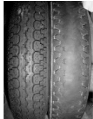
*Some tires have wear bars, that is, rows of nubs that are recessed into the spaces between the treads. If any portion of a tire's tread is worn down to level with the wear bars, it is time to replace the tire. The tire on right is well past that point.*
