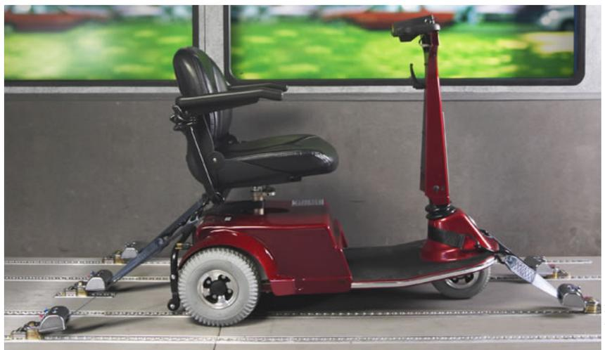
*Q'Straint recommends that securements for 3-wheeled scooters flare out wider in the back than in the front.*
