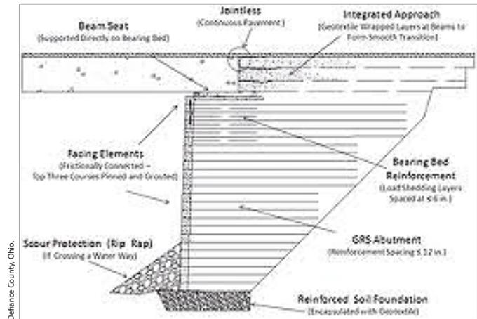
Typical cross section of a GRS-IBS abutment face wall.
