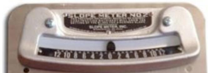
Figure 3. A slope meter accurately displays the percent of cross slope.
