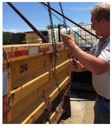
Out of the rack and back on the truck: Wilson attached a chain to the ring on the back of the tailgate and pulls on the hoist's chain hand- over-hand to shorten it and lift the tailgate out of the rack.
