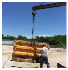
Manoeuvering the tailgate is easy once the chain supports it. The boom moves freely and the tailgate can be positioned where needed.
