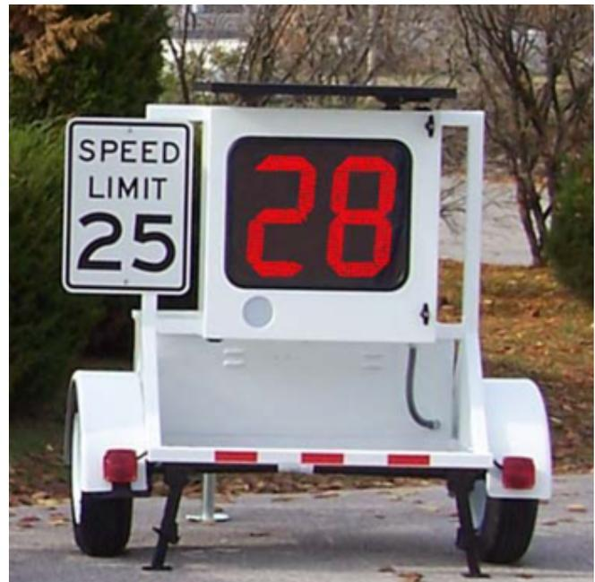
Figure 1: Radar Speed Trailer (2)
