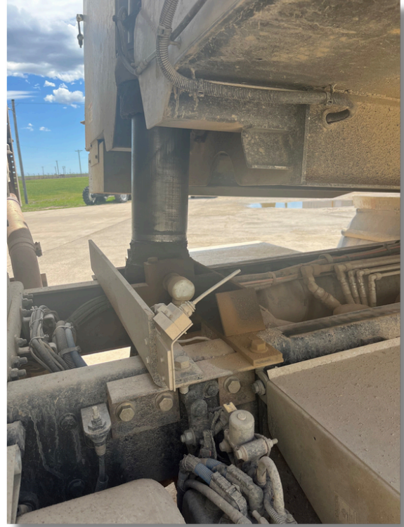
Sensor has lost contact with the bed. Photo credit: Darren Fishel
