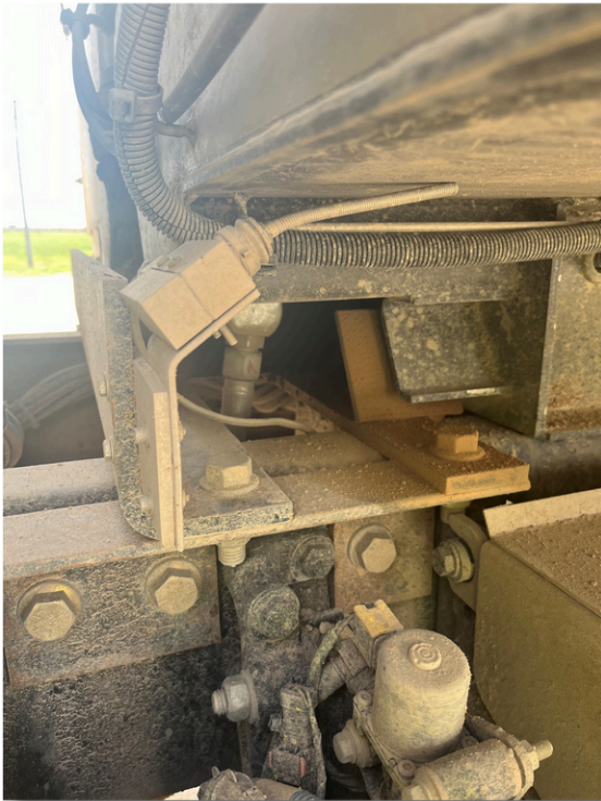
Sensor in contact with the bed. Photo credit: Darren Fishel
