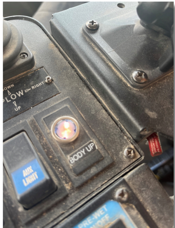
In-cab Body Up indicator. Photo credit: Darren Fishel
