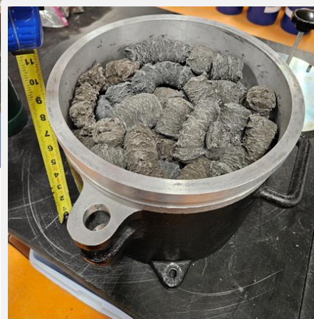
Resin8 in 0.5 f 3 mold after confined compressive strength test
