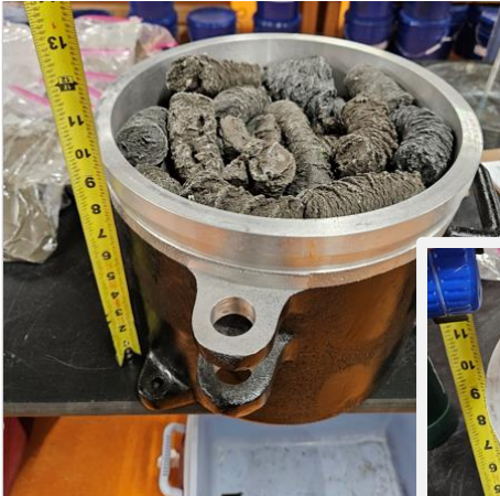
Resin8 in 0.5 f 3 mold before confined compressive strength test
