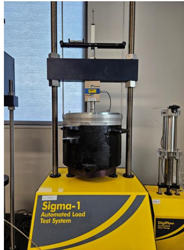
Resin8 in testing mold setup on load frame during Consolidation test
