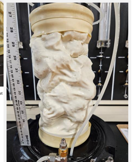
Resin8 in membrane after CID test
